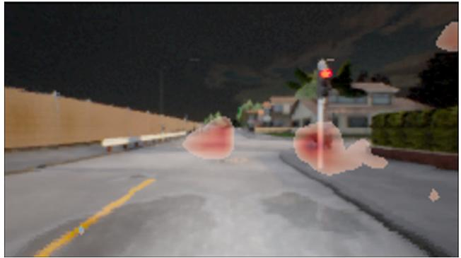
Fig. 2: Saliency map generated by using blur-based saliency (details: Sec. III-A) for the pre-trained Learning by Cheating IL model [18]. The center input image to the model is shown with saliency overlaid. This scene depicts the instant a vehicle comes to a stop after which it fails to restart. Notably, the bulk of saliency weight is at the traffic light’s base — a non-causal region which indicates causal misattribution.
